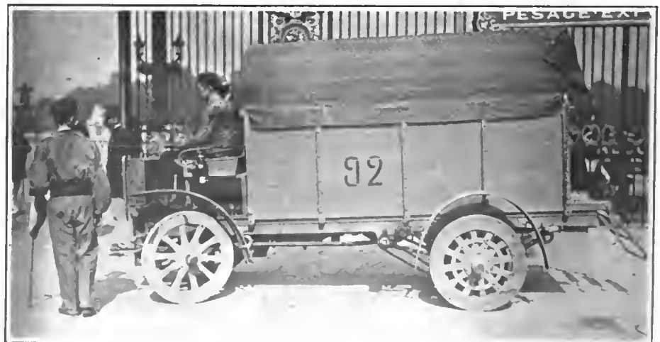
ARIEL GASOLINE ARMY WAGON CARRYING ABOUT 2,700 POUNDS IN FRENCH TRIALS
